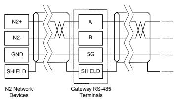
Figure 25: N2 Bus Cable Connection
